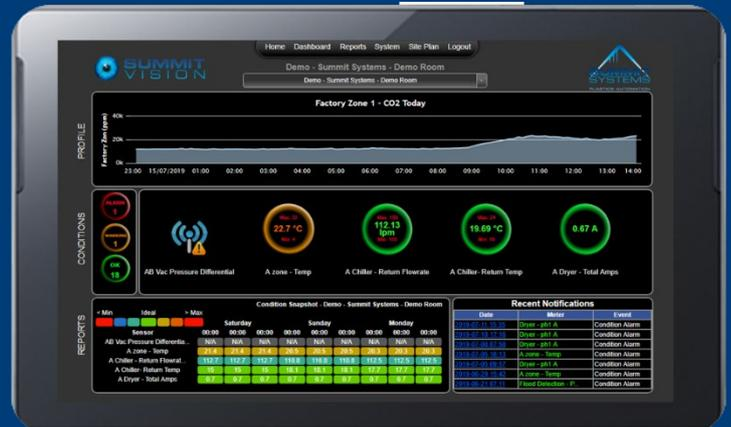
After 30 minutes of user familiarisation, the customer set some preliminary alert thresholds, making the system fully operational. The principle is straightforward; aside from on-screen alerts, emails and texts are sent to nominated users when a data reading goes out of normal parameters.
