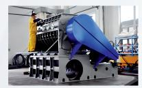
Granulators can be tailored to fit various applications, for example with oversized suction troughs in order to achieve a very high output.
