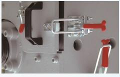
The Quick Snap System allows the lower front plate section to be easily removed for granulator cleaning. The lower front plate section is held in position by two sturdy lever clamps.
