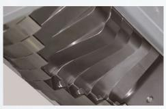
Staggered rotor blades creates an individual blade cut thus increasing the cutting torque. All of the machines in this series are therefore suitable for grinding more solid materials and thicker walled sprues.
