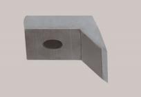
The curvature of the specially profiled rotor knives ensures a constant cutting radius after re-sharpening thus maintaining the original cutting gap. Awkward knife adjustment is no longer necessary.
