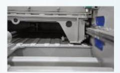
The ZCS system uses a sturdy roller guided drawer type ram to feed the material into the shredder. Seamented cutting chamber and ram allow trouble free processing of thin materials.
