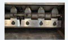
The granulator part uses a sturdy F+ rotor to ensure a good ingestion of the material flow while still being able to handle thicker and heavier particles.
