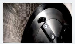
PM Pulverizers can be equipped with either one piece, or segmented grinding discs. Discs are made from high quality tool steel and can be treated to withstand longer wear.
