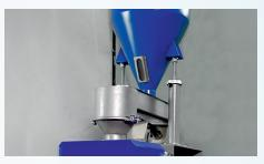
Material is fed into the pulverizer by a vibrating dosing channel, the feeding rate is automatically adjusted based on the motors amperage and material temperature.
