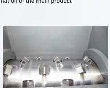
The internal ram design on the ZIS series allows the cutting chamber volume to be increased while keeping a small footprint. Making the ZIS ideal for shredding of big volume parts.
