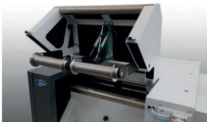
Independent pneumatic dancing arms for each roller.
