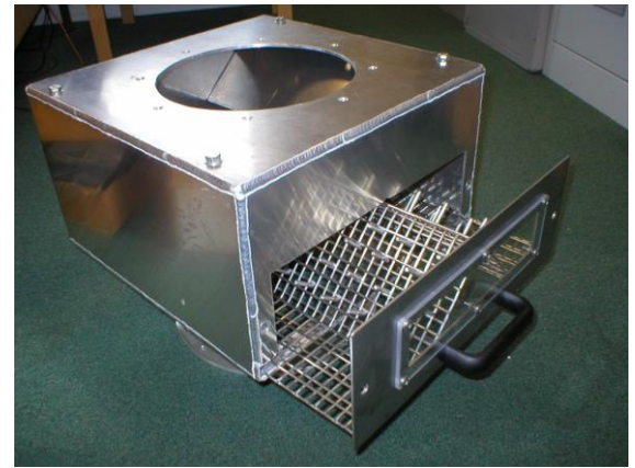
Day bin box with drawer in open position
