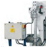
Hopper opening with motorized jack and screen-holder opening by gas cylinder.
