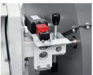
Rotor lock for maintenance. Safety devices and circuit in compliance with EEC Directives.
