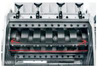
Rotary discs integral with the rotor and rings. Arrow cutting configuration for grinders with 3 or 5 blades; bench adjustment of blades and counterblades.
