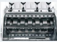
Rotary discs integral with the rotor and rings. Arrow cutting configuration for grinders with 3 or 5 blades; bench adjustment of blades and counterblades.
